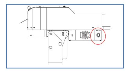
Cut off the power supply and clean the remaining paper inside. If you cannot clean the paper from the outlet, open the flap to clean it.
